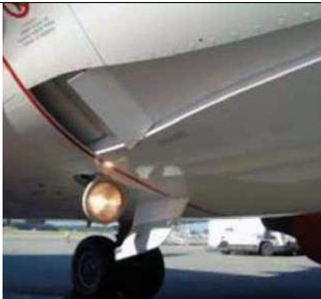
Figure 6. A ram air door controls the flow of air through the primary and secondary heat exchangers
