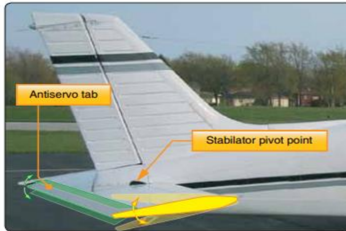
Figure 1-76. An antiservo tab moves in the same direction as the control tab. Shown here on a stabilator, it desensitizes the pitch control.
