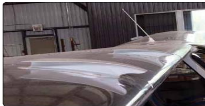
Figure 1-79. The Symphony SA-160 has two unique vortex generators on its wing to ensure aileron effectiveness through the stall.
