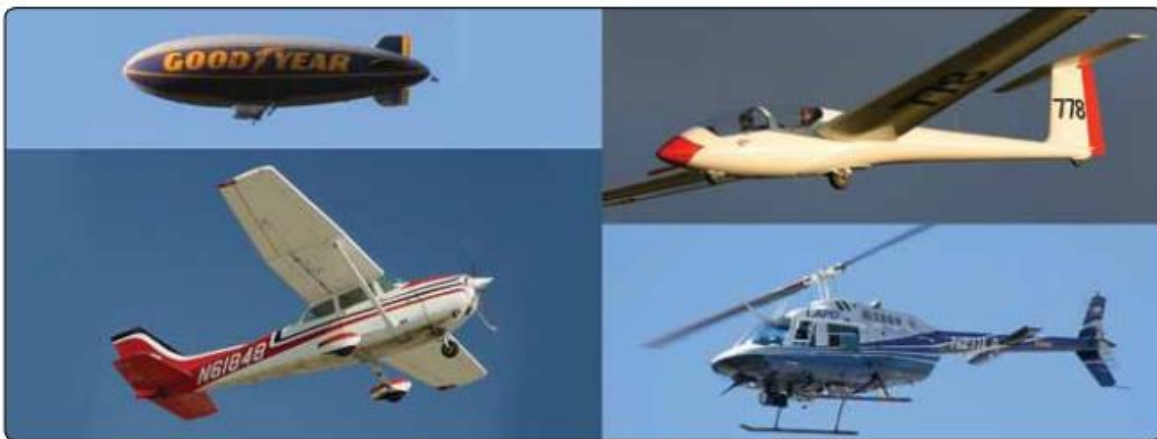
Figure 1-11. Examples of different categories of aircraft, clockwise from top left: lighter-than-air, glider, rotorcraft, and airplane.
