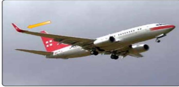
Figure 1-77. A winglet reduces aerodynamic drag caused by air spilling off of the wing tip.
