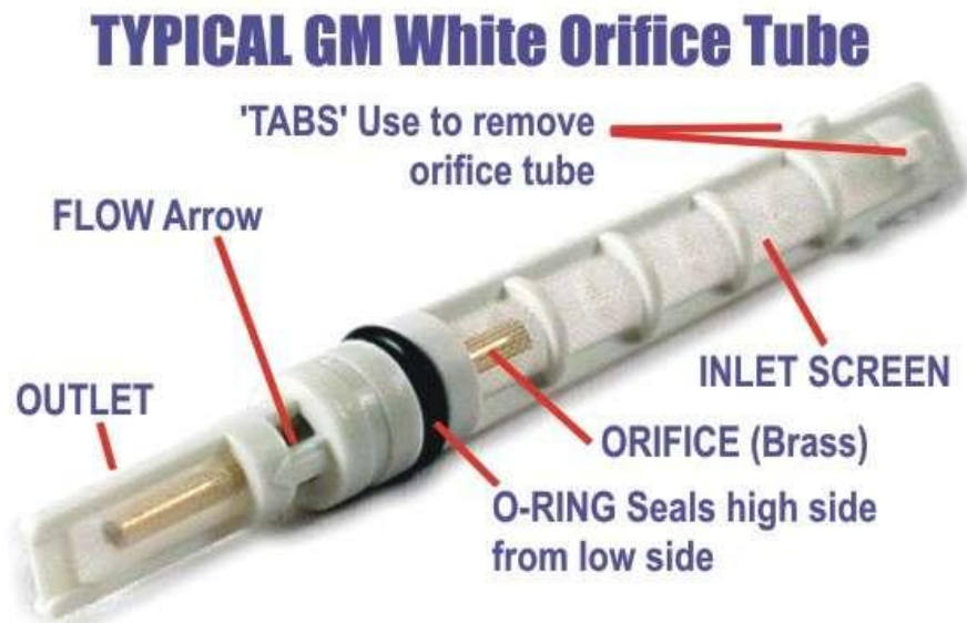
Figure 3 orifice tube details
